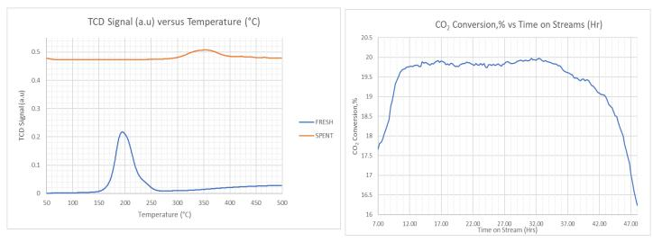
Figure 2 TPR Profile for fresh and spent Cu/Zn/Al/Zr catalyst sample
