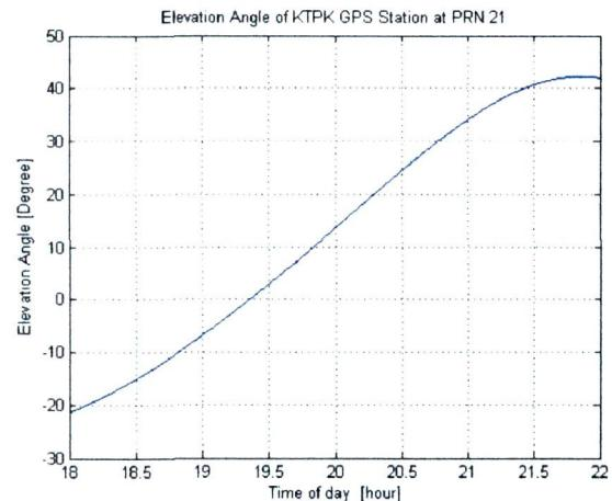
Figure 6: Graph of elevation angle against time
