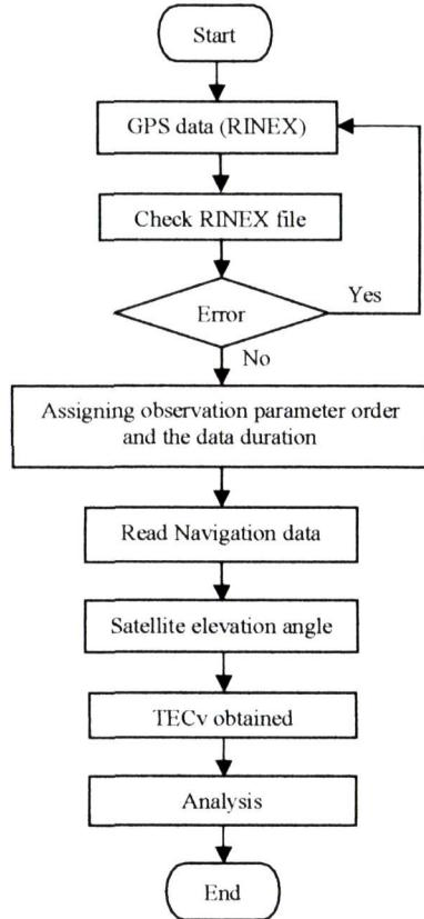
Figure 3: Flowchart process in TEC processing
