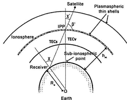
Figure 2: Geometry of Satellite-Receiver Link
