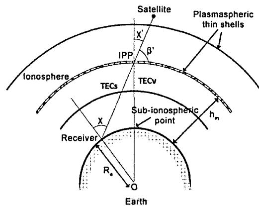
Figure 2: Geometry of Satellite-Receiver Link
