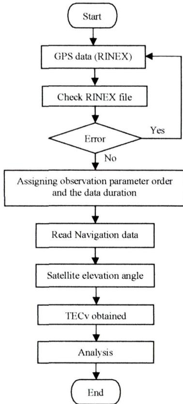
Figure 3: Flowchart process in TEC processing
