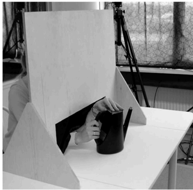
Fig. 3 Experiment setup where the participants could only touch the product without the influence of vision (Dagman et al., 2010).
