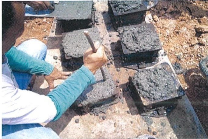
Photo 3.31: The concrete was poured into the mould for test cubes.
