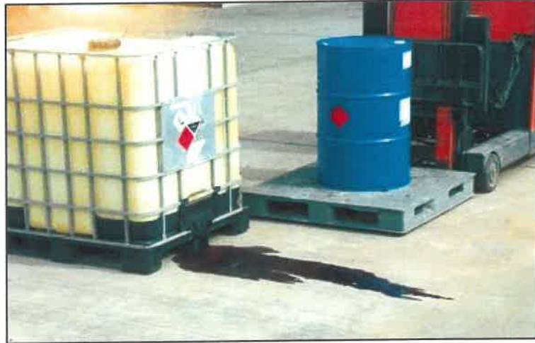
Figure 9: leaks on the container
