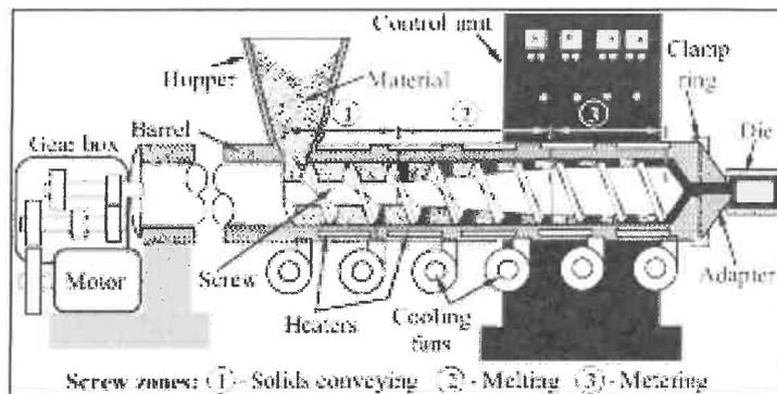
Figure 4.7 Single Screw Extruder Diagram Working Principle
