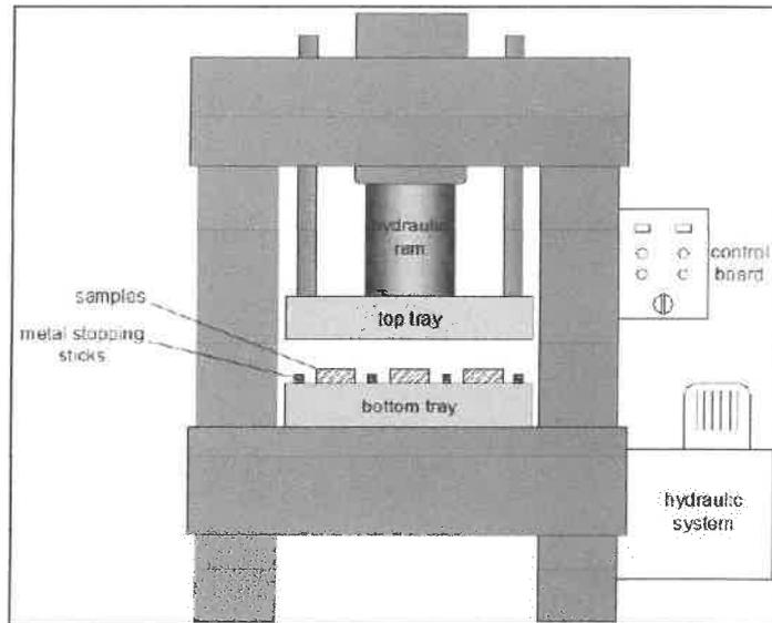
*Figure 4.9 Working Principle of Hot-press*
