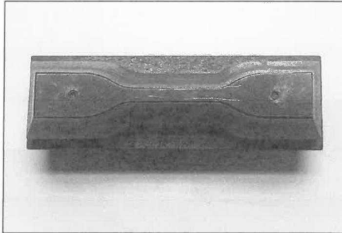
Figure 4.14 Dumbbell shape ASTM D638 Type IV
