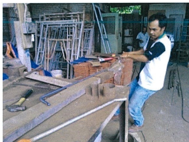
Figure 3.8 The forming process of RC bars
