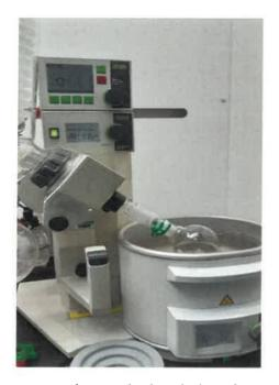
Figure 2: the water vapor to extract the standards solutions from 80 ml to 5 ml concentrated
