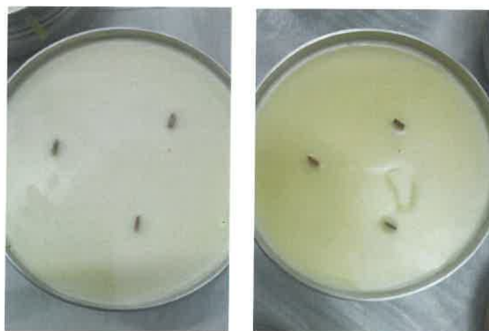
Figure 4.13: The candle has a crack and bubbles on the surface during trial run experiment
