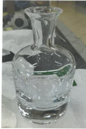
Figure 4.4: Result of clean glass after using detergent, hot water, tap water and some other tools
