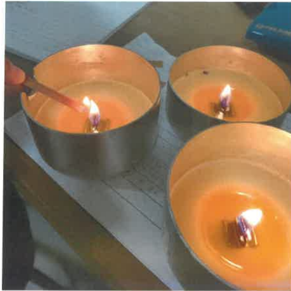
Figure 4.16: Burning the candle form a tunnel
