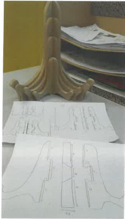
Figure 4.5: Examples of roughly drawing of wood stand with actual dimension before transferred to Rhinoceros
