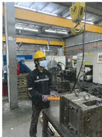
Figure 4.5.2. PPE during lifting and install/uninstall mold using crane
