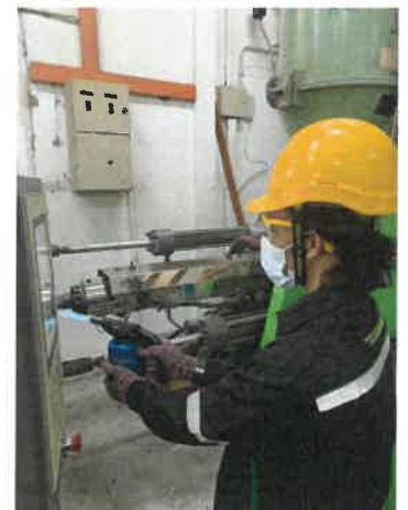
Figure 4.5.3. PPE during applying external heating on nozzle.
