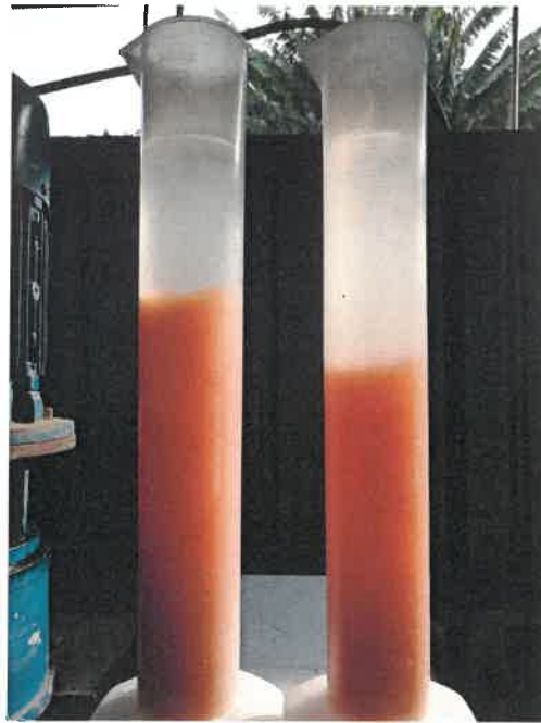
Figure 5: Photo taken from 19 th May 2022 with average SVI value 650ml (Left: from aeration tank 2, Right: from aeration tank 1)
