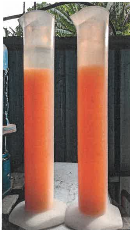
Figure 6: Photo taken from 26 th June 2022 with average SVI value 865ml (Left: from aeration tank 2, Right: from aeration tank 1)
