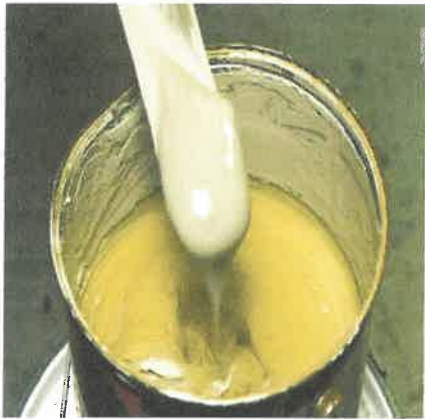
Figure 22: The sedimentation of the solid constituents comprising pigments and extenders
