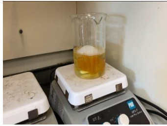
Figure 3: The mixture mixed using a hot plate and a PSTE magnetic stirrer
