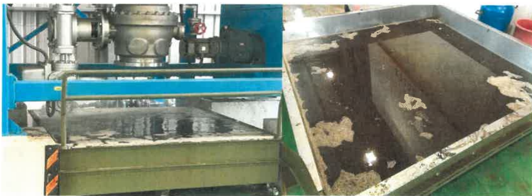
Appendix 4: Final product of the fish waste after SCW process. Comes out in liquid form.
