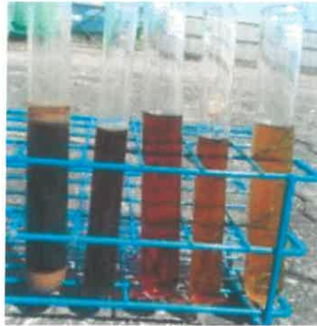
Left to right: raw POME, coagulation with 10mL, 2mL, 30mL and 40 mL Ferric Chloride.
