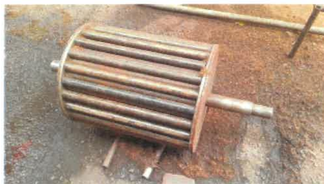
Figure 29: Rotor of ripple mill
