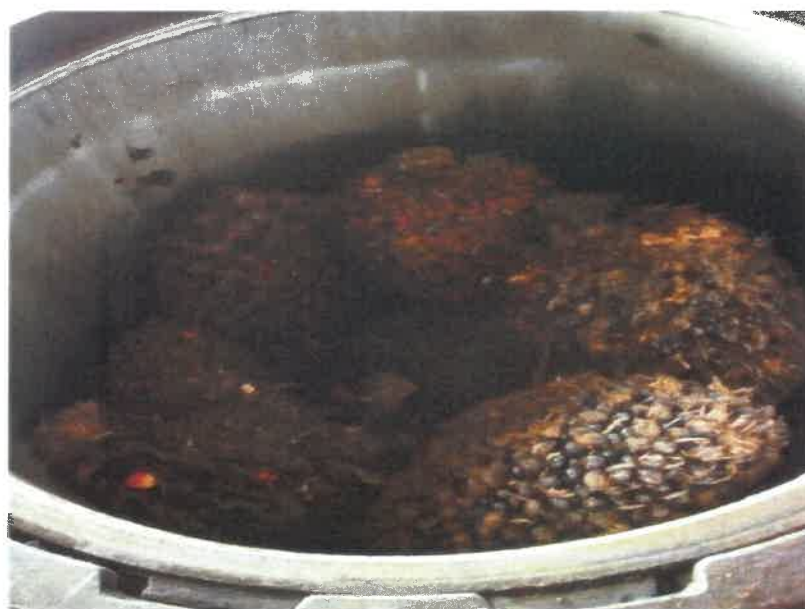
Figure 37: The condition of FFB in the sterilizer
