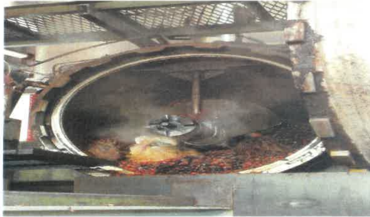
Figure 38: The bunch in the sack that will be taken out of sterilizer
