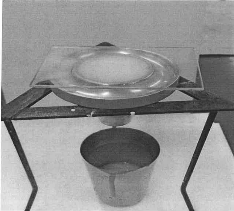
Figure 4.2.2.6 Example of glass on the DIN cup
