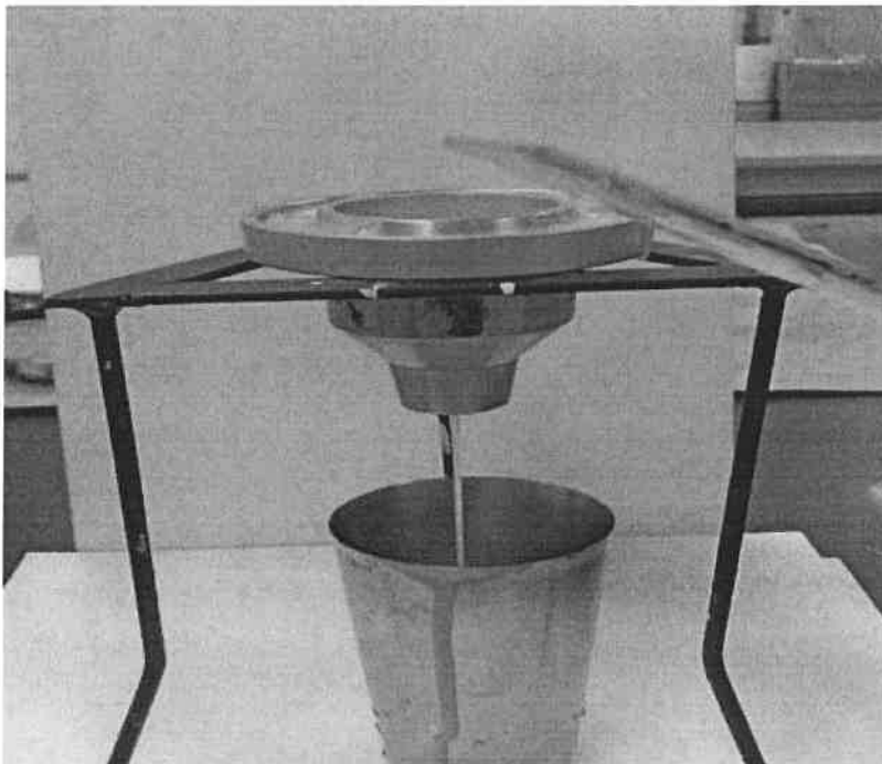
Figure 4.2.2.7 Example of viscosity test
