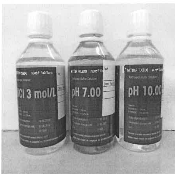
Figure 4.2.2.29 buffer solutions From left to right: KCl storage solution, buffer solution pH 7 and buffer
