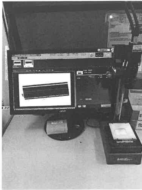
Figure 12: Computer with tool stack height master software and measurement camera
