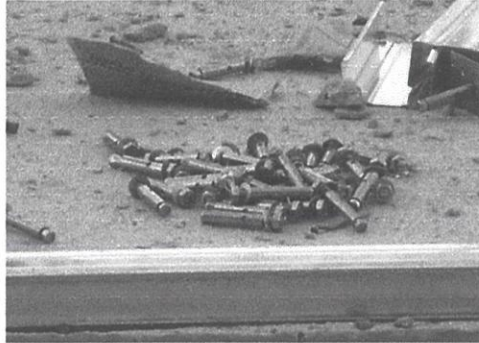
Gambarfoto 4.3c: P. J Anchor (E- 1076- B) - wall plug
