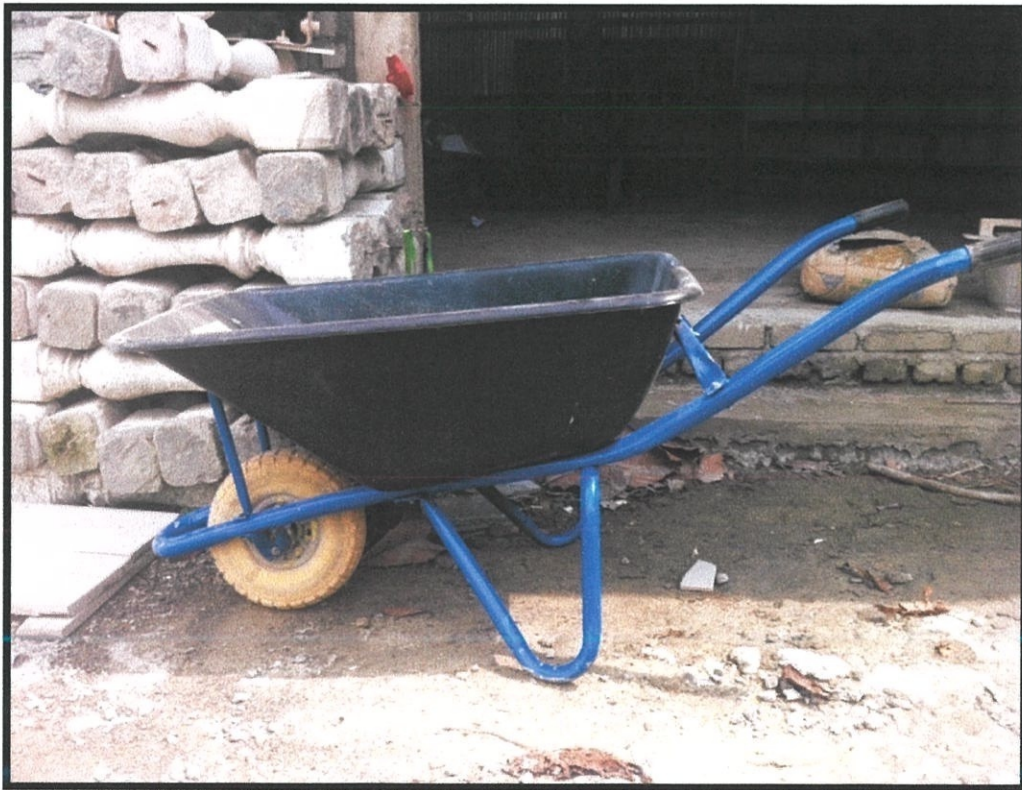
Figure 3.14: Wheelbarrow used to bring brick and other material.
