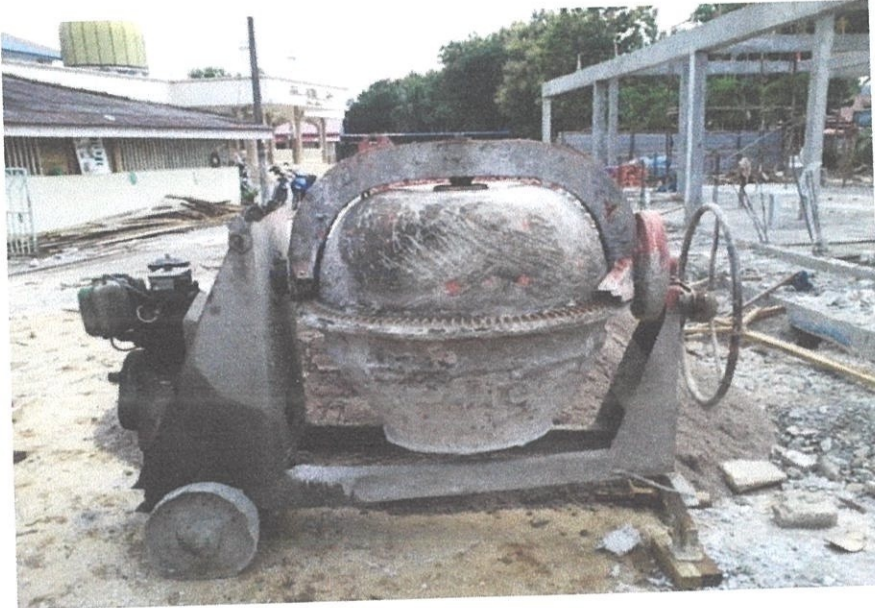
Photo 3.16 Concrete mixture usually use to make in small quantity of concrete
