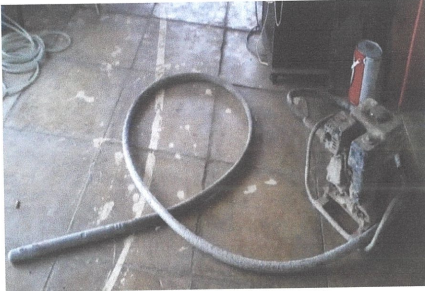
Photo 3.17 Vibrate the concrete produce a strength and higher density of concrete
