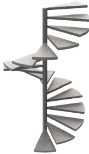
Picture 1.3 : Spiral stairs
