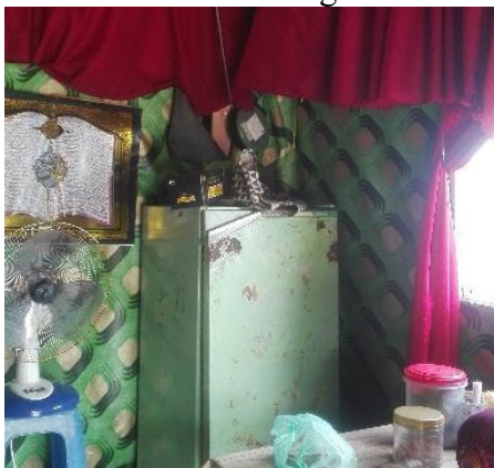
Corrosion of electrical equipment and door hinge
