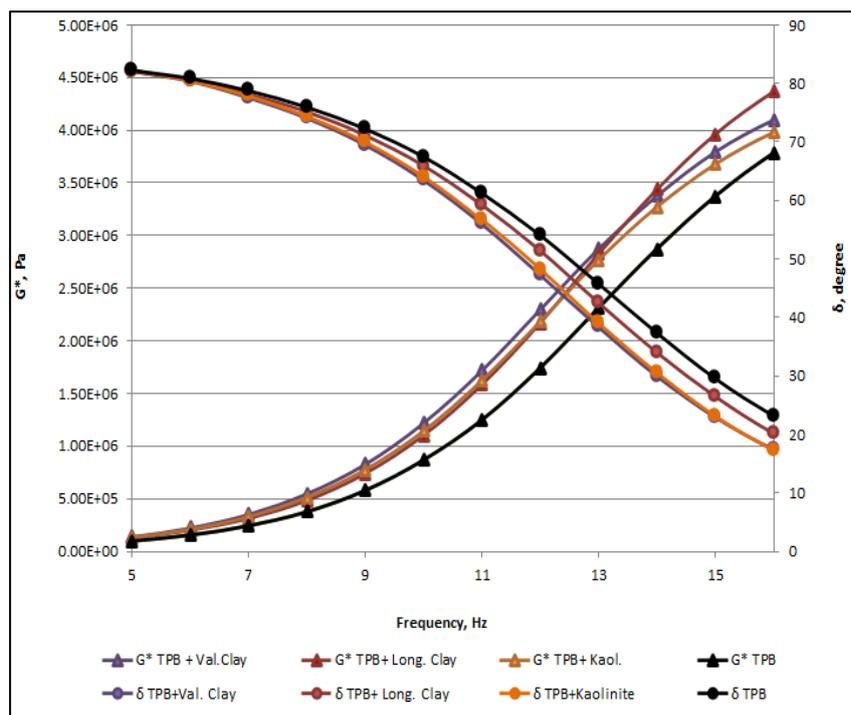
**Figure 3.** The effect of clay source on the rheological properties of TPB blends (20% clay additions) at 323 K.
