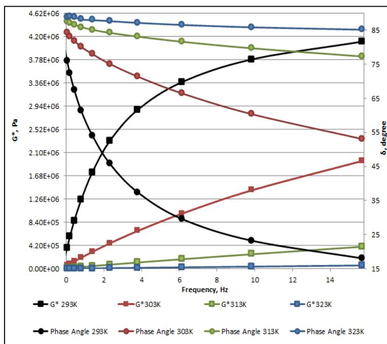
**Figure 1.** The effect of temperature and frequency on the rheological properties of TPB.
