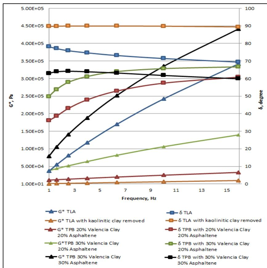
**Figure 5.** The effect of adding Valencia Clay and asphaltenes on the rheological properties of TPB at 333 K.
