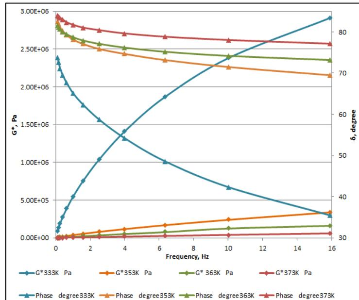
**Figure 2.** The effect of temperature and frequency on the rheological properties of TLA.
