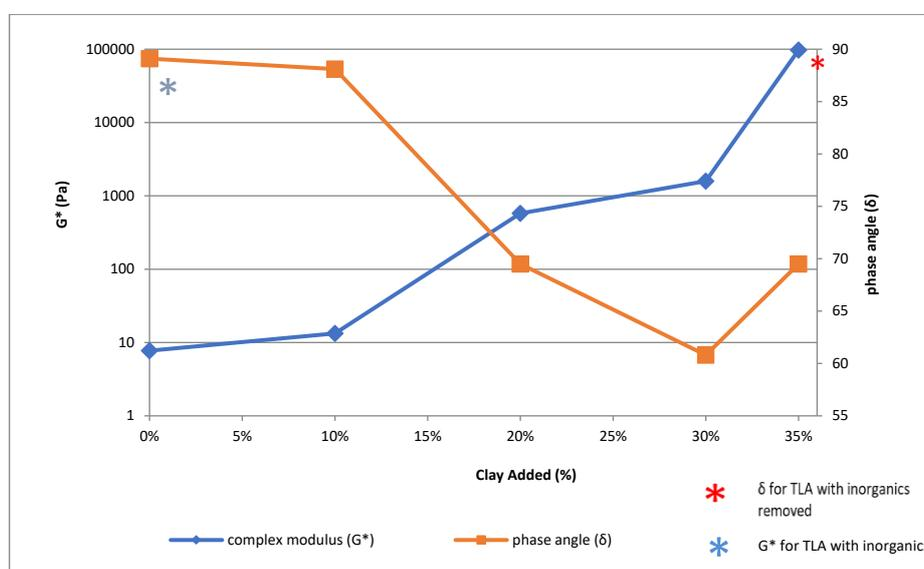
**Figure 4.** The effect of the % clay content on the rheological properties of complex modulus ( $G^*$ ) and the phase angle ( $\delta$ ) at 333 K at a shear stress of 24 Pa.
