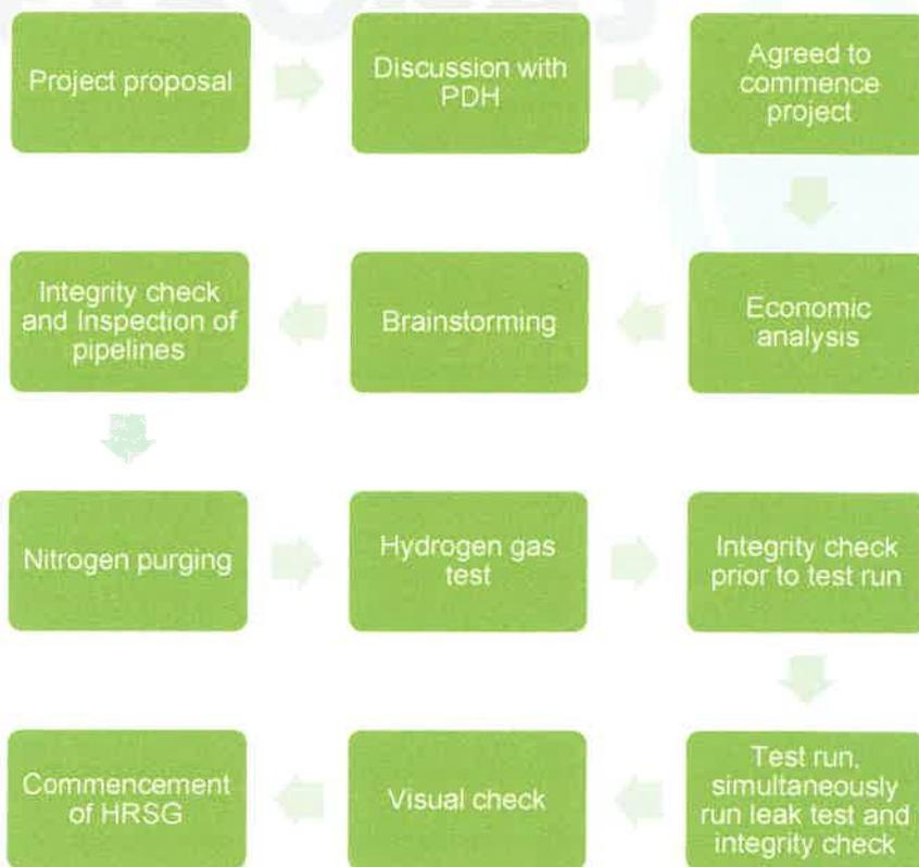
Figure 37 Flow chart for Reinstating H<sub>2</sub>RG system supply from PDH project
