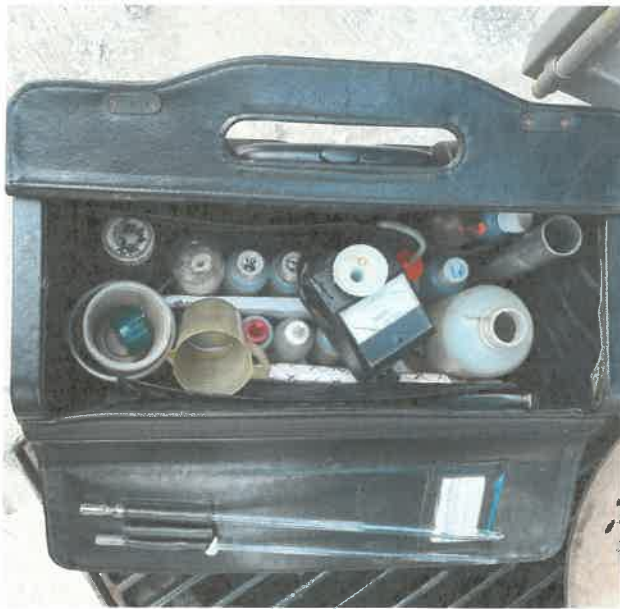
Figure 3: Water testing kit for boiler water quality analysis
