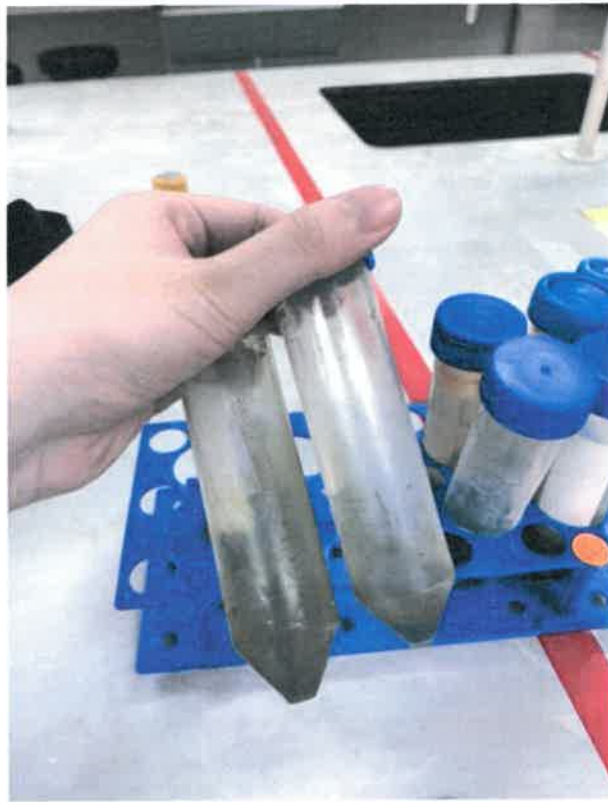
Figure 28. 2 nd method making nanoparticles where agglomeration took place
