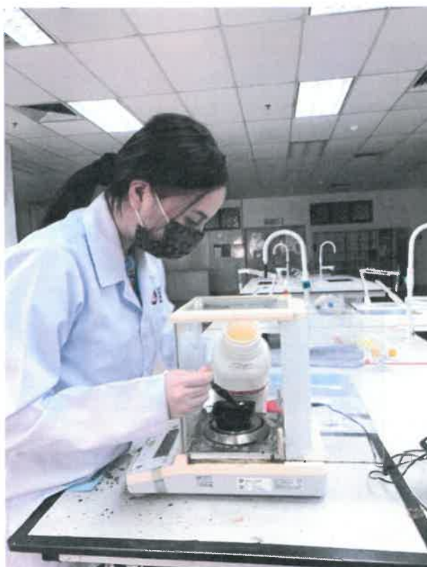
Figure 6. Measuring Polyvinylpyrrolidone, Copper (II) Acetate and Silver Nitrate using analytical balance
