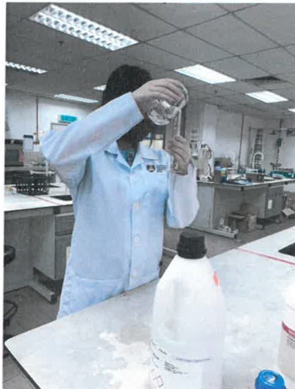
Figure 7. Measuring Ethylene Glycol solution using beaker and measuring cylinder
