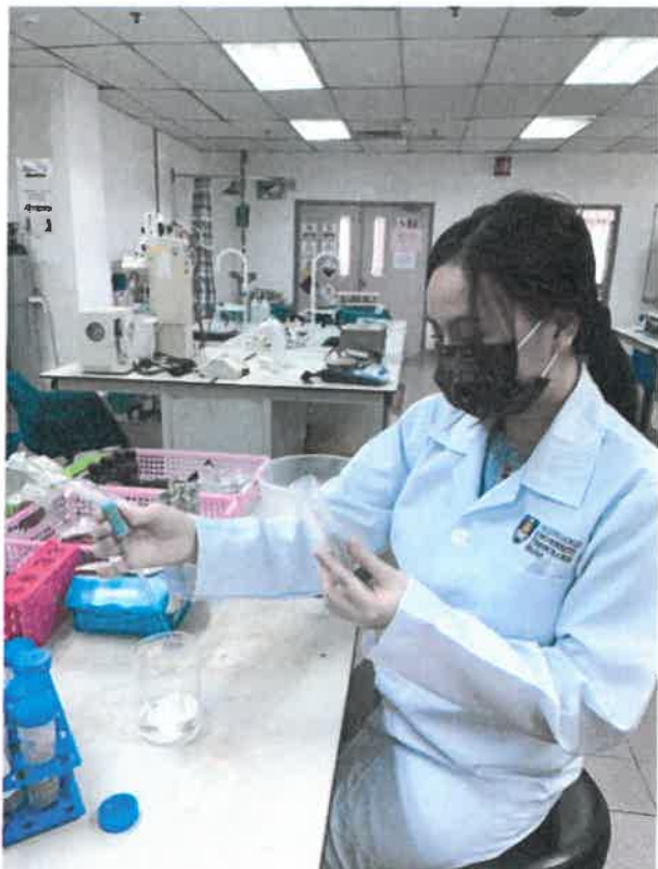
Figure 11. Removing excess unwanted liquid from the nanoparticles formed
