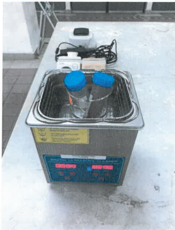
Figure 9. Cooling the reagent with water bath (Digital Ultrasonic Cleaner)
