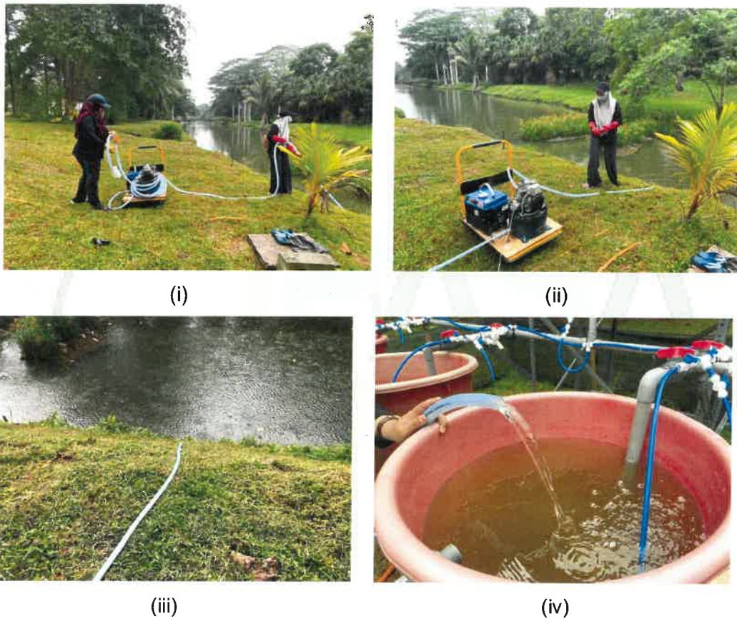
Figure 3.8: (i); (ii); (iii); (iv) Water Filling from Lake into The Tank
