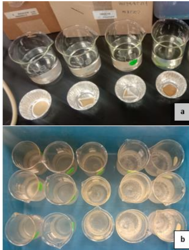
Figure 5. Beaker holding filtered water before drying (a) Residue (TDS) after the oven-dried process(b)
