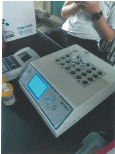
Figure 7. COD test on the treated water at Matrix Flavours & Fragrances Sdn. Bhd.
