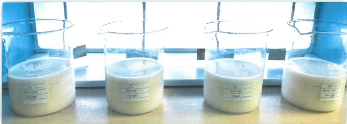
Figure 11. Result shown from left is RM10-4005, RM10-3001, RM10-5001 and RM10-2009 after 1 hour of settling time.
