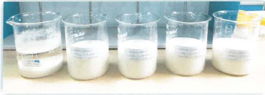
Figure 12. From left is when lime powder was added with lime and the remaining beakers are when there is no lime powder added.
