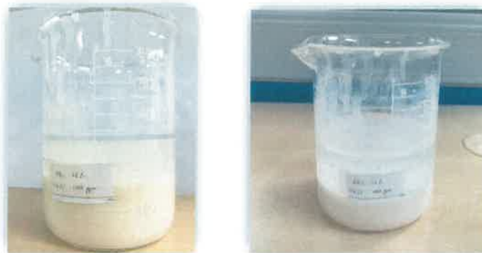
Figure 13. Comparison between 30 minutes and 1-day settling time for the chemical usage of PAC 16%.
