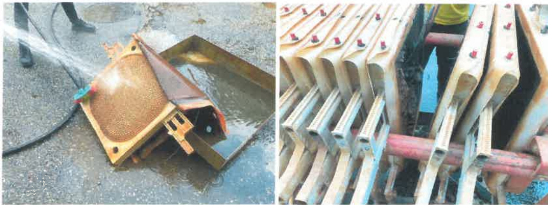
Figure 18. Cleaning process of filter press equipments.
