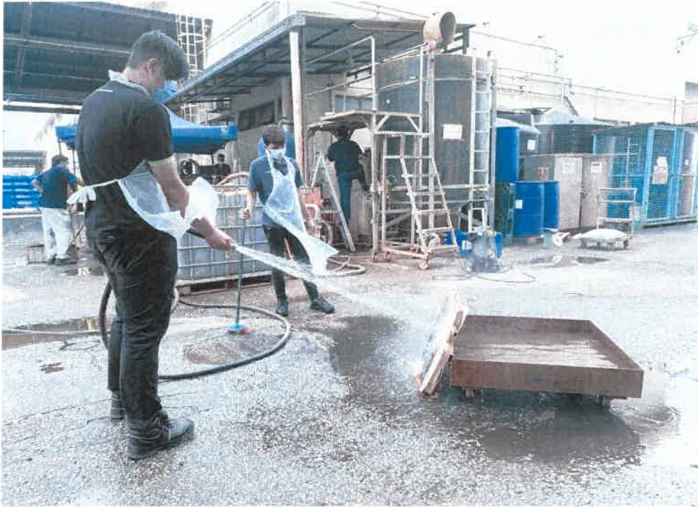
Figure 21: Cleaning the block of the filter press
