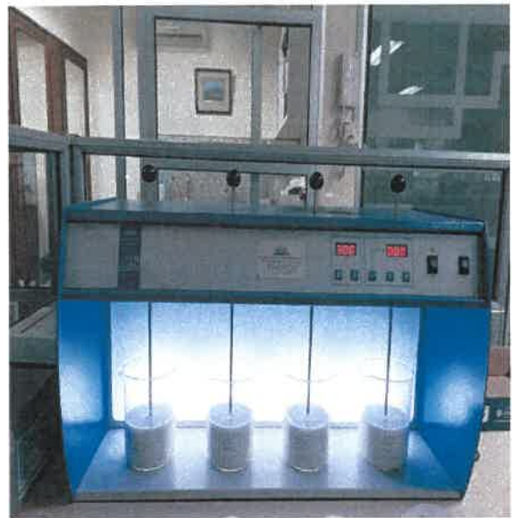
Figure 30: Performing jar test for Vnotion's project
