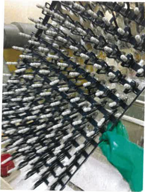
Figure 12: Aluminium spool during etching
