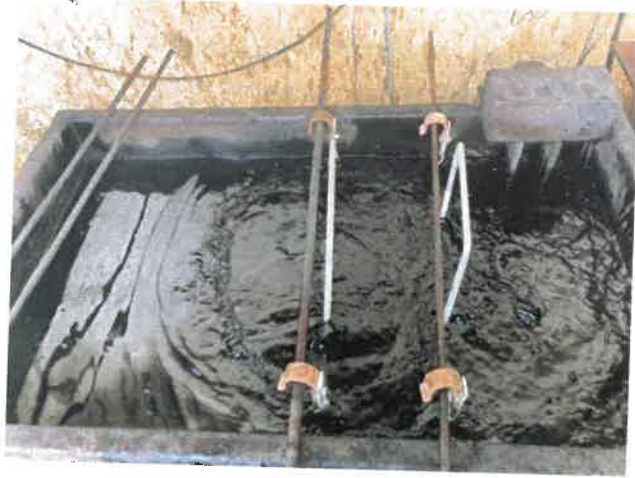
Figure 16: Carbon treatment ( Teflon plating line) (offline tank)
