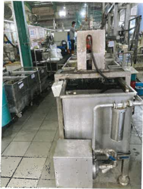
Figure 14: Electroless nickel plating line
