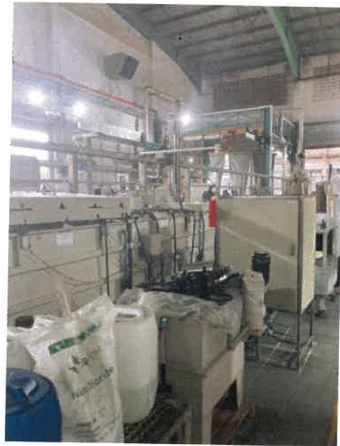
Figure 15: Teflon/pure zinc plating line (right)
