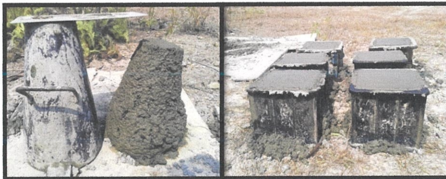
Photo 3.13 Slump test and cube test
