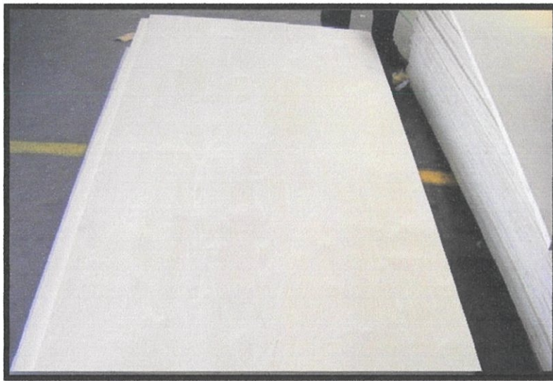
Photo 3.14 Plywood used to make formwork
