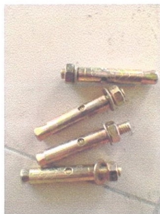
Photo 3.18: The Wall plug used to support Aluminum track
