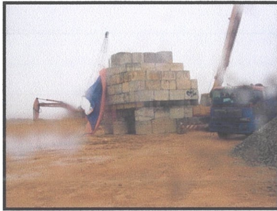
Gambarfoto 4.5: Ujian Maintained Load Test (MLT)
