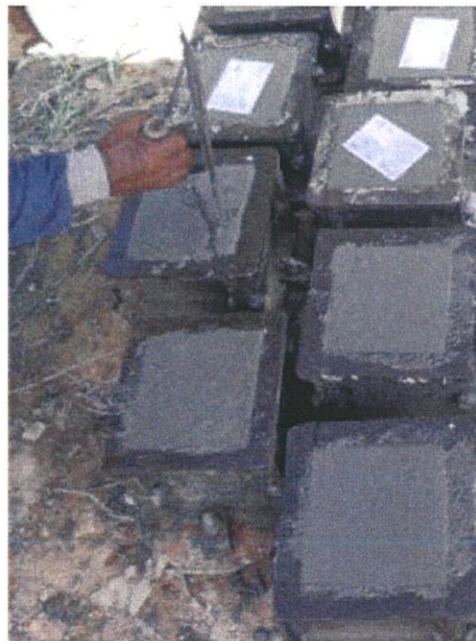
Photo 3.16 Set of cubes for cube test
