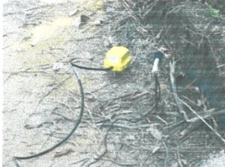
Figure 3.7 Seismograph is placed on the ground.(Draw-off tower)
