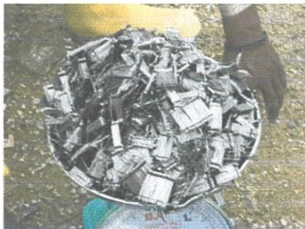
3.31 Measuring weight of steel fiber. (Valve House)
