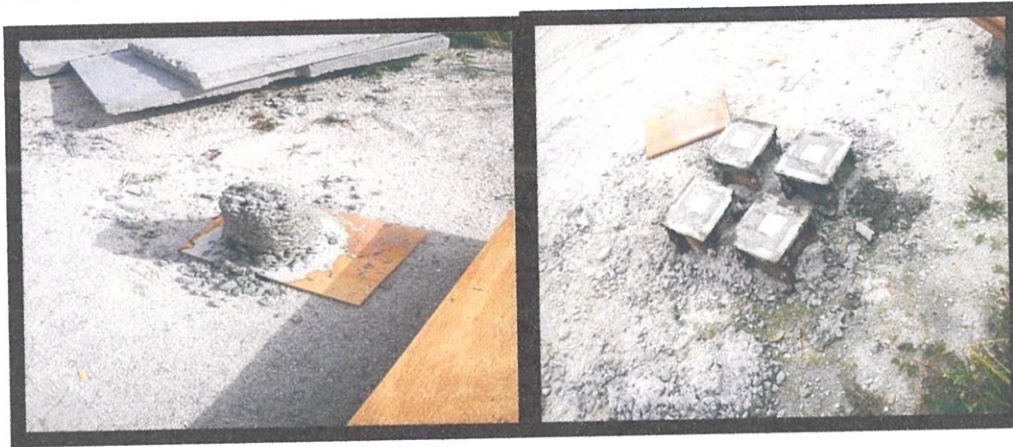
Photo 3.16: The cube test of the concrete
