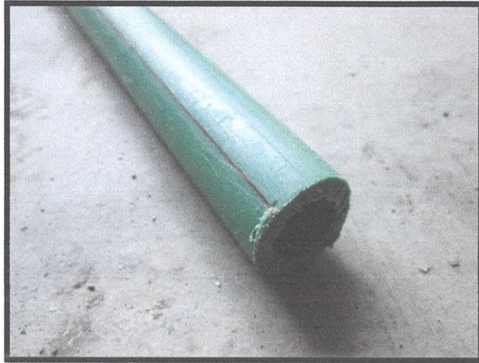
Photo 3.1 PPR pipe for hot water
