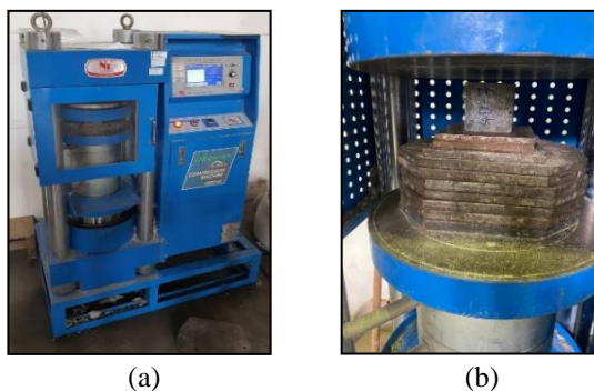
Figure 4: Image of (a) compression test machine, and (b) cube specimen
