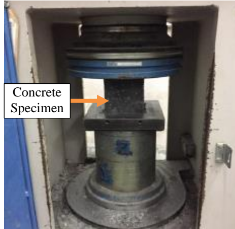
Figure 1: The specimen after compressive test
