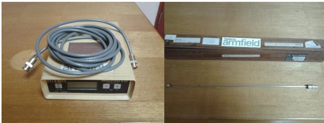
Figure 3.6: Current meter equipment to measure the stream velocity.
