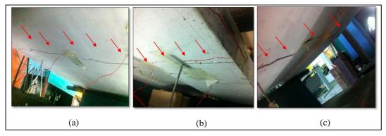
Figure 7: Mode of failure of all samples; (a) solid-SFRC, (b) rib-SFRC, (c) rib-SFRC-GFRP
