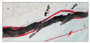
Figure 6: Steel fiber bridging the cracks of concrete
