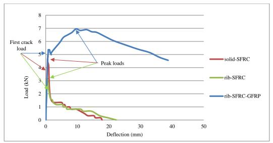
Figure 4: Load versus deflection of the samples
