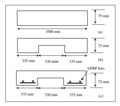
Figure 3: The cross section of (a) solid-SF (b) rib-SF and (c) rib-SF-GFRP
