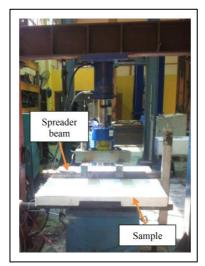
Figure 3: Sample tested under three-point load set-up
