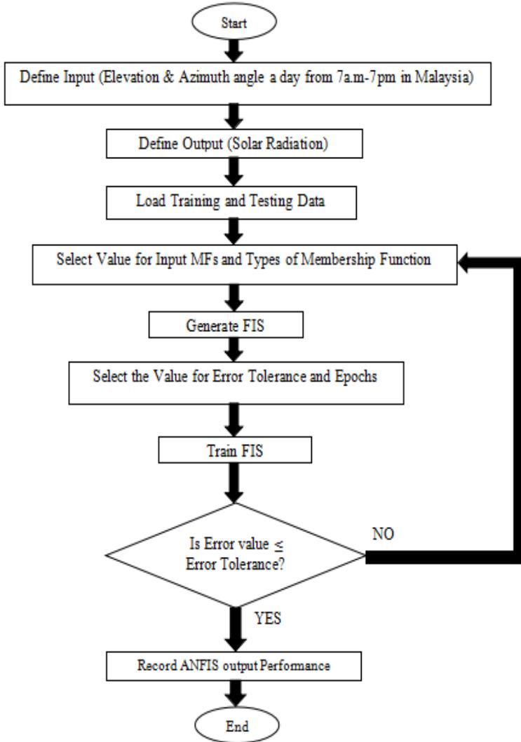
Figure 2: Flowchart for ANFIS dual axis solar tracker
