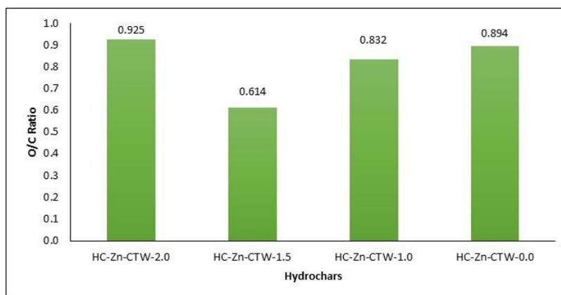
Figure 2: O/C ratio for hydrochars obtained at different  $ZnCl_2$  loading
