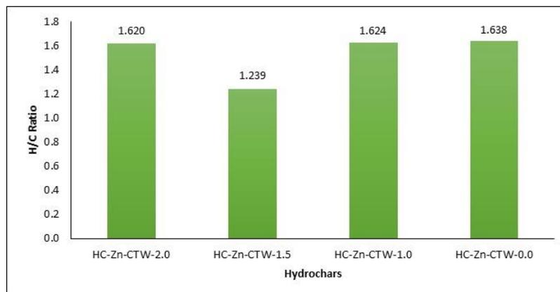
Figure 1: H/C ratio for hydrochars obtained at different  $\text{ZnCl}_2$  loading
