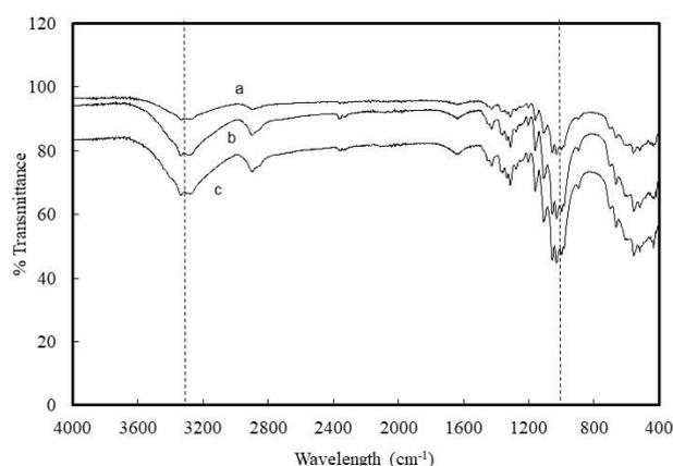
Figure 3: FTIR spectra for hydrochars obtained at different  $ZnCl_2$  loading (a) HC-Zn-CTW-2.0, (b) HC-Zn-CTW-1.0, (c) HC-Zn-CTW-1.5
