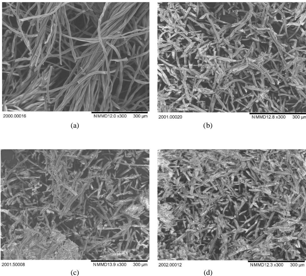
Figure 4: SEM images of (a) HC-Zn-CTW-0.0 at 300X magnifications, (b) HC-Zn-CTW-1.0 at 300X magnifications, (c) HC-Zn-CTW-1.5 at 300X magnifications, (d) HC-Zn-CTW-2.0 at 300X magnifications
