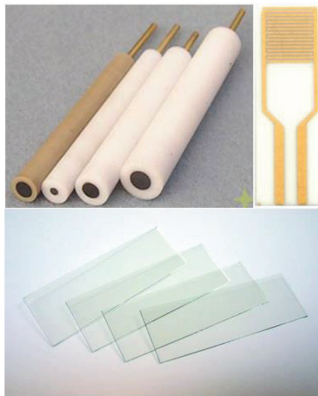
Figure 4. Frequently used electrode substrates. The top left is the GCE, the top right is the AuE, and the bottom is the ITO.
