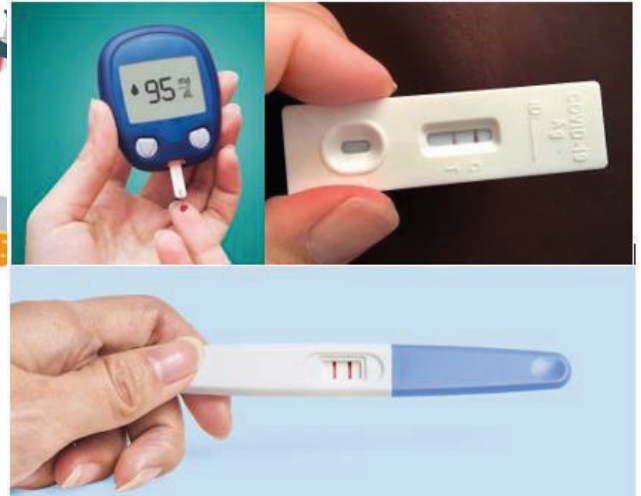
Figure 1. Commonly used biosensors. The top left is the glucose biosensor, the top right is the COVID-19 rapid test kit, and the bottom is the pregnancy test kit.
