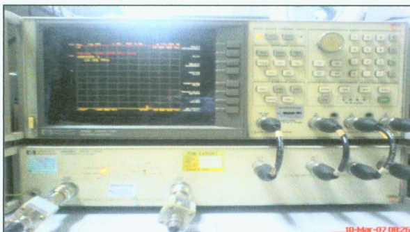
Figure 6: HP 8753C 300Khz-3GHz network analyzer and HP 85046A 300Khz - 3.0GHz S-Parameter Test Set .
