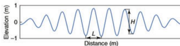
Figure 1: Definition for wave height and length
