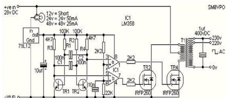
**Figure 2.** Energy conversion circuit
