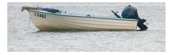
Figure 1.2 Example for Glass Reinforced Plastic boat with an outboard engine.
